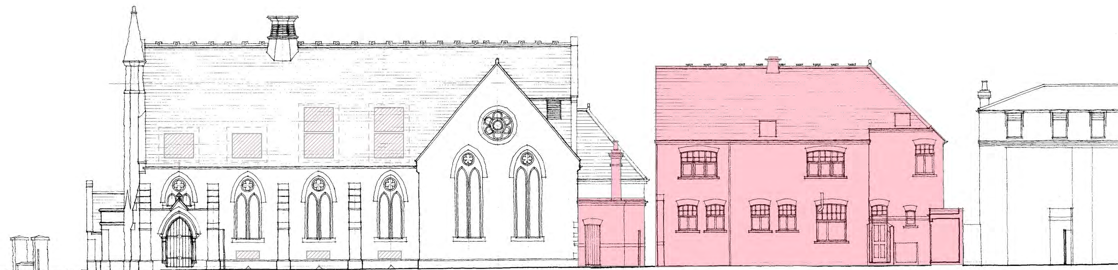
Demolitions North Elevation
