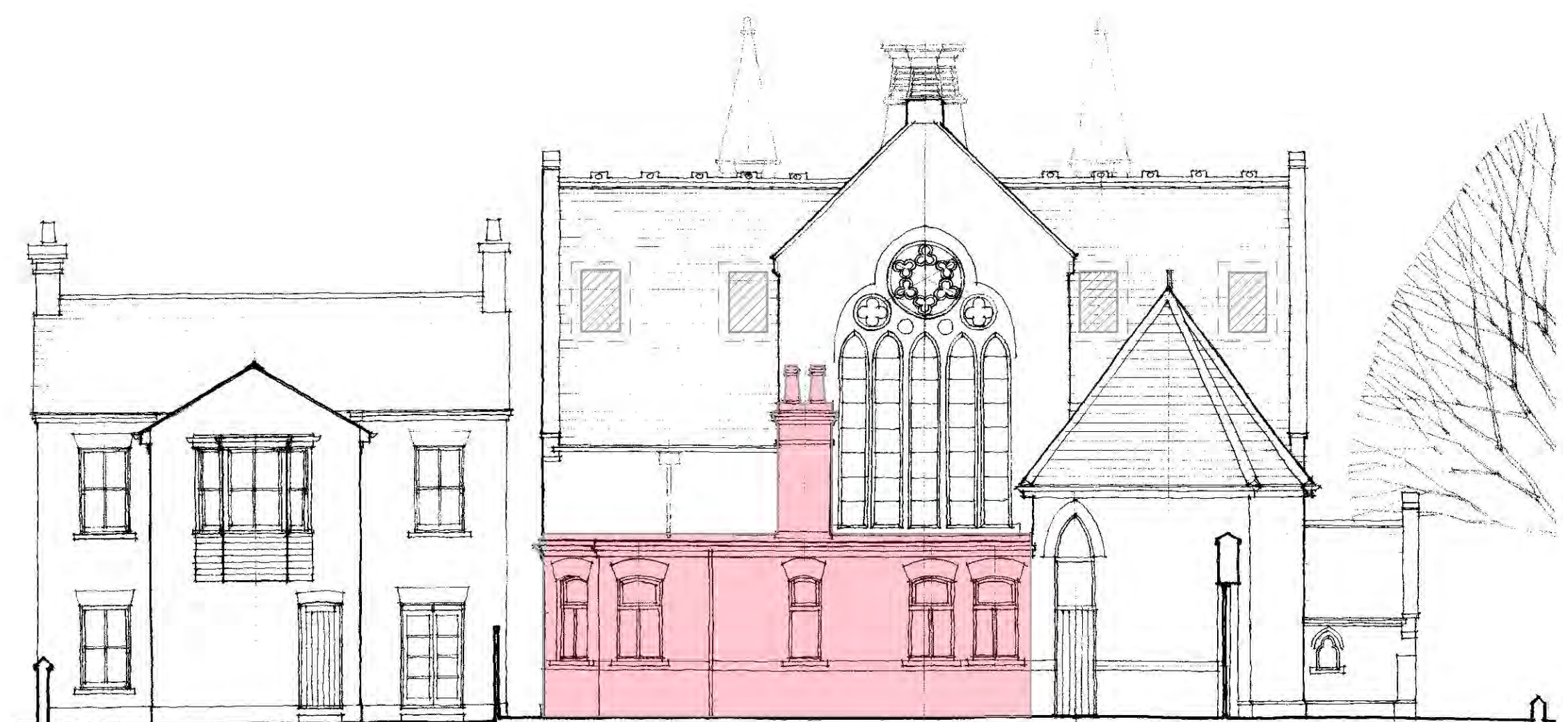
Demolitions West Elevation
